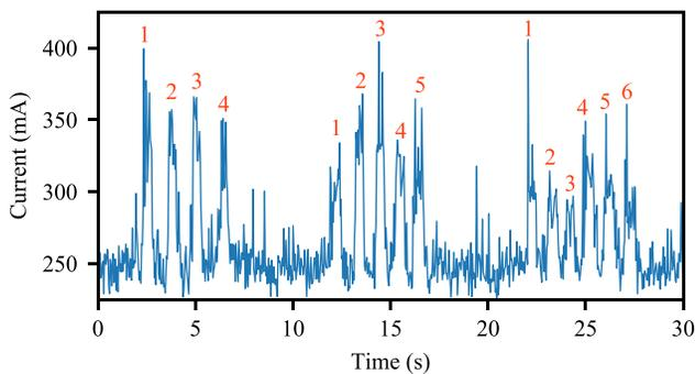
**Figure 12: The wireless charging current trace reflecting the input of three passcodes of lengths of 4, 5, and 6 digits. A few seconds of inactivity separate the entry of each passcode. Each digit corresponds to a momentary surge in current draw.**
