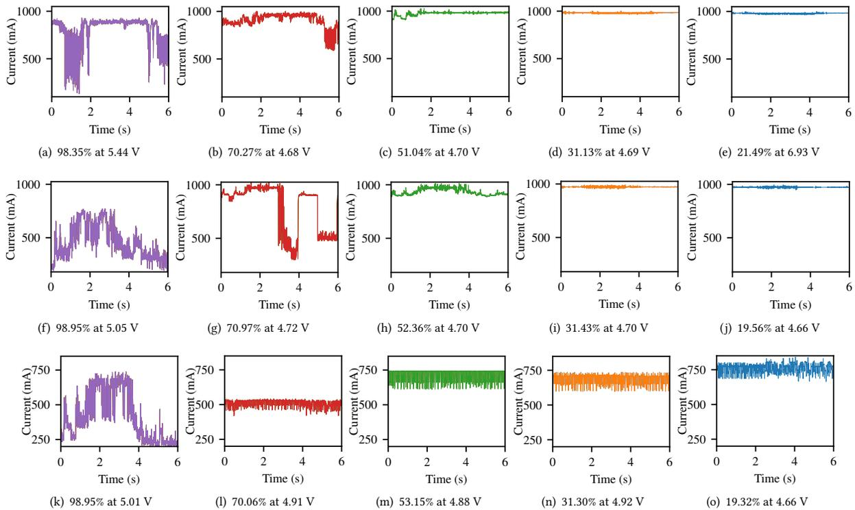
**Figure 11: Current traces for loading zoom.us on different devices while wirelessly charging and USB charging: wired iPhone 6s (top), wired iPhone 8 (middle), wireless iPhone 8 (bottom).**
