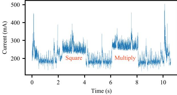
**Figure 14: The current trace that demonstrates distinction between idle time and repeated square/multiply operations.**
