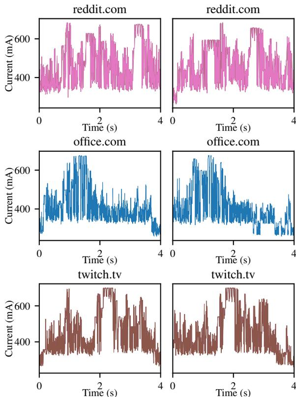
**Figure 5: Current traces demonstrating the activity leaked when automatically loading webpages on an iPhone 11.**
