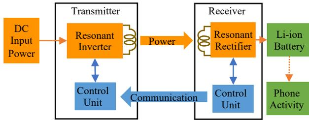
**Figure 1: Transmitter and receiver hardware for the Qi standard.**
